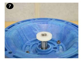
B It may be easier to thread the molded in bolt into the shaft if the diaphragm(s) is inverted on one or both sides. This can be done by hand. • The other diaphragm(s) (items 21/22) and inner/ outer plates (items 20 & 23) can be installed onto the opposite end of the shaft (item 32).
