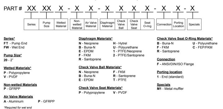
**Example Pump P/N's**: FT20P-PP-RRPR-F1, FT20P-PA-BBPB-F1, FT20V-PP-1TVC-F1 & FT20V-PA-FFVF-F1 **Example Wet End P/N's**: FW20P-RRPR, FW20P-BBPB, FW20V-1TVC & FW20V-FFVF
