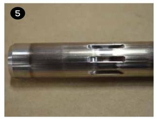
• After determining if the condition of the shaft is acceptable, ensure both center section o-rings (items 33 & 34) are in place on both sides of the center section.
