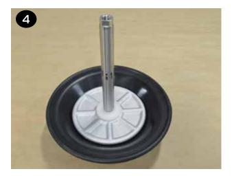
• The shaft (item 32) and shaft o-rings (item 30) should retain the lubricant that was factory applied. If they appear dry, apply a light coat of lithium thickened grease. Avoid over lubrication as it can cause decreased performance of the air distribution system.
