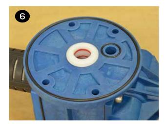
Install both air chambers (item 26) by placing one side on top of the center section (item 35). Ensure the air path hole of the center section lines up with the through hole in the air chamber. Insert the bolts & washers (items 24 & 25) through the air chamber and center section. • Flip the components over and place the remaining air chamber on the center section. Thread the nuts & washers onto the bolts (items 24, 25 & 40). Tighten and torque the fasteners.
