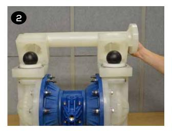
**3** Repeat the above steps for the suction manifold (item13). The seat o-rings, valve seats and valve balls (items 14, 15, 16, & 17) are located in the liquid chambers (item 19).
