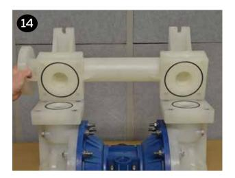
Stand the pump upright onto the suction manifold feet (item 13). Place the large o-rings (item 15) into the glands in the face of the liquid chambers (item 19) followed by the small o-ring (item 14) in the gland of the valve seats (item 16). Place the valve seats on the liquid chambers with the o-ring down against the liquid chamber.
