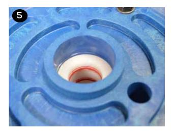
• Push the shaft (item 32) through the center of the shaft bushing (item 29). It is normal for this to be a tight fit, especially if the shaft and shaft o-rings (item 30) are in good condition.
