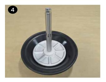
• The shaft (item 32) and shaft o-rings (item 30) should retain the lubricant that was factory applied. If they appear dry, apply a light coat of lithium thickened grease. Avoid over lubrication as it can cause decreased performance of the air distribution system.
