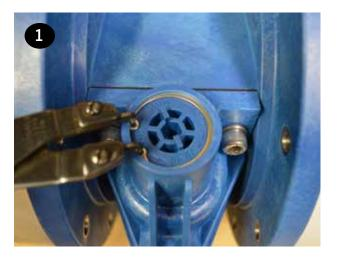
• Aluminum Air Valve - To replace the valve cap o-rings (item 5), remove the (3) button head cap screws (item 7) using a 5mm hex wrench. Repeat for the remaining cap.
