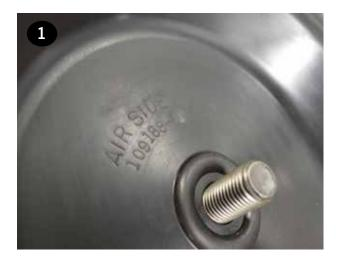
Place the inner plate (item 23) over the molded-in bolt. Ensure the round recess in the plate faces the diaphragm (item 22).
