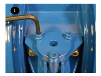
Plastic Air Valve - Remove and replace o-ring (item 5). Install cap (item 6) and tighten until groove for the retaining ring is visible. Install retaining ring (item 8). **Aluminum Air Valve** - Remove and replace o-ring (item 5). Install cap (item 6), tighten, and torque the valve cap screws (item 7). Repeat for the remaining cap.
