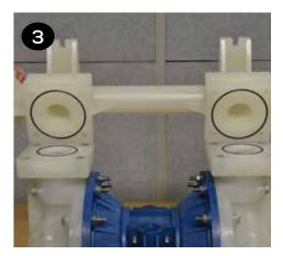
Remove both liquid chambers by removing the (12) bolts, washers & nuts (items 11, 12, 18 & 27) on each liquid chamber using a 17mm wrench and nuts can be removed using a 15mm wrench. Inspect and replace diaphragms if needed. • To remove the diaphragms (items 21/22), begin by loosening the (2) outer plates (item 20) using two 30 mm wrenches. Use 6-sided sockets or wrenches to prevent damage to the hex portion of the outer plate.
