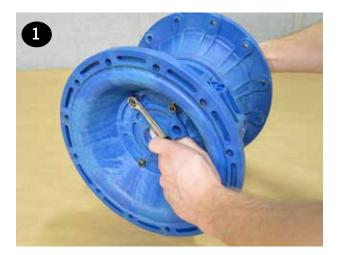
Remove and set aside the air valve (item 3) using a 6 mm hex wrench (see "Valve & Muffler Gasket Replacement" section for more details). The shaft bushings (item 29) can be removed by placing a large socket between the two bushings. Place an extension into the socket from one side of the center section. Tap with a rubber mallet to remove the bushing. Repeat for the remaining bushing.
