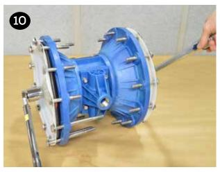
**Note**: When installing polytetrafluoroethylene (PTFE) diaphragms, it is important to tighten outer plates simultaneously (turning in opposite directions) to ensure tight fit.
