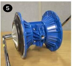
Remove the outer plate, diaphragm(s), and inner plate (items 19, 21/22 & 23) from the side that is loosened. Pull or push the shaft (item 32) and remaining plates and diaphragms out of the center section. If pulling, it may be easier to grip the diaphragm if it is inverted.
