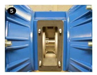
**6** Tighten and torque the (4) cap screws & washers (items 1 & 2) into the muffler plate.
