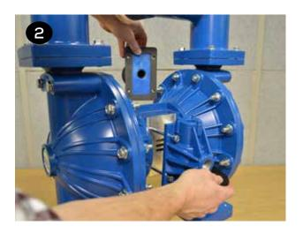
3 Place the new gasket (item 38) on the air valve (item 3) and ensure the slots in the gasket align with the slots in the air valve and valve plate (item 10).
