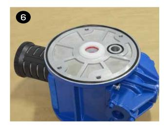
Install air chambers (item 26) by placing one side on top of the center section (item 35). Ensure the air path hole of the center section lines up with the through hole in the air chamber.
