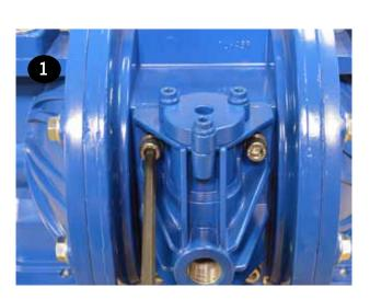
Pull the valve body and gasket (items 3 & 30) off the front of the center section (item 28) and the muffler plate gasket, muffler plate and muffler (items 29, 31, & 33) off the back.
