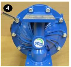
To remove the diaphragms (items 20/21), begin by loosening the (2) outer plates (item 18) using 2-30mm wrenches. Use 6-sided sockets or wrenches to prevent damage to the hex portion of the outer plate.
