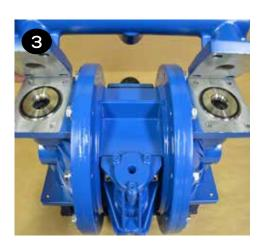
Remove both liquid chambers (item 17) by removing the (10) bolts (item 16) on each liquid chamber using a 13mm (or ½") wrench. Inspect and replace diaphragms if needed.
