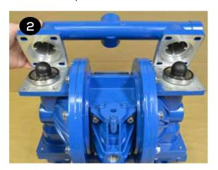
Repeat the above steps for the suction manifold (item12). The seat o-rings, valve seats and valve balls (items 13, 14, & 15) are located in the liquid chambers (item 17).
