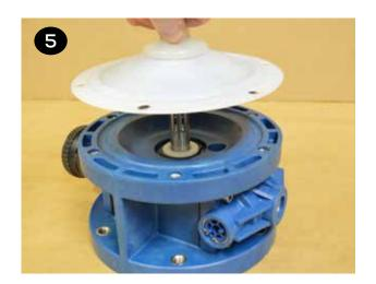
The other diaphragm(s) (items 20/21) and inner/outer plates (items 18 & 22) can be installed onto the opposite end of the shaft (item 27). It may be easier to thread the bolt into the shaft if the diaphragm(s) is inverted on one or both sides. This can be done by hand.
