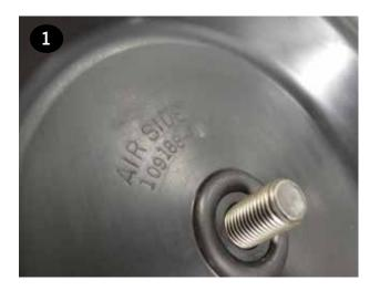
Place the inner plate (item 22) over the cast/threaded bolt. Ensure the round recess in the plate faces the diaphragm (item 21).
