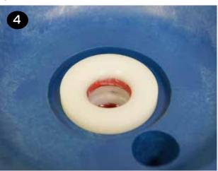
Drush the shaft (item 27) through the center of the shaft bushing (item 24). It is normal for this to be a tight fit, especially if the shaft and shaft o-rings (item 26) are in good condition.
