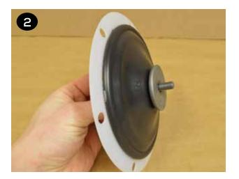
Apply a couple drops of a medium strength thread locker, such as Loctite® 246, to the molded in outer plate bolt (item 19). Thread the shaft (item 27) onto the molded in bolt until it is snug to the flat back side of the inner plate (item 22).
