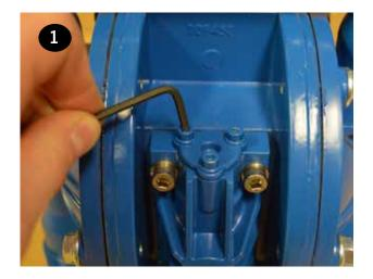
Plastic Air Valve - Remove and replace o-ring (item 5). Install cap (item 6) and tighten until groove for the retaining ring is visible.
