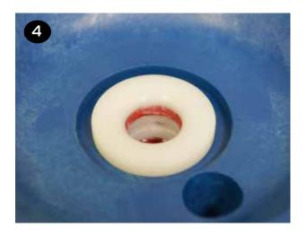
• Push the shaft (item 27) through the center of the shaft bushing (item 24). It is normal for this to be a tight fit, especially if the shaft and shaft o-rings (item 26) are in good condition.
