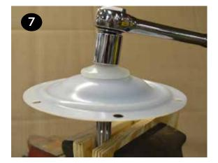
After performing required maintenance, the pump can be reassembled. The pump can also be reassembled using the disassembly instructions in the reverse order as listed above. For detailed assembly instructions, follow steps Wet End Reassembly instructions on next page.
