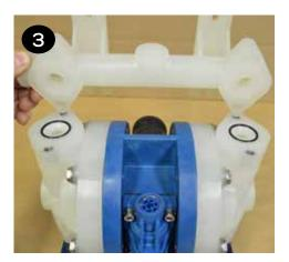
• Remove both liquid chambers by removing the (6) bolts (items 17) on each liquid chamber using a 13mm (or ½") wrench. Inspect and replace diaphragms if needed.
