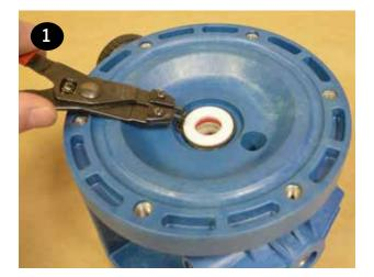
**C** Use the supplied grease packets to lightly grease the OD and ID o-rings (items 23 & 26) that come preinstalled in the new shaft bushing supplied in air end kits.
