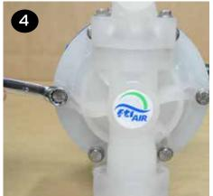
• To remove the diaphragms (items 20/21), begin by loosening the (2) outer plates (item 19) using 2-20mm wrenches. Use 6-sided sockets or wrenches to prevent damage to the hex portion of the outer plate.
