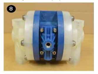
• Flip the pump upside down and drop the suction valve balls (item 16) into the liquid chamber (item 18) ball cages.
